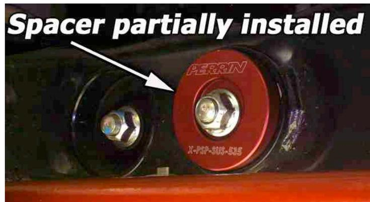
10. Continue threading nut/stud into diff cover until differential is pulled up to subframe. You will feel the increase in tension on nut when this happens. Continue threading nut until roughly 70-ft-lbs of torque is felt on nut. **NOTE: Because you are pressing Lockout bushing into subframe using bolts, some popping may occur. When step is complete, PERRIN Lockout bushing will be sticking out from subframe .125" to .25".**
