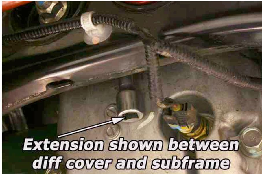
13. Tighten nut/stud into diff cover while holding 3/8" extension in place. Tighten nut to 50ft-lbs. When step is completed, PERRIN lockout bushing will be flush or slightly concave with subframe.
